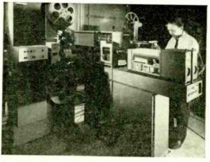
film density whilst electronic circuits compensate for film dye imperfections. The system has been designed by Marconi with the exception of the film projection mechanisms which are of well-established professional manufacture. A sync. interlock drive motor is employed which allows precise registration of separate magnetic sound followers. The equipment is intended for use with a Westrex sound follower unit, but other units may be employed providing minor modifications are made.
